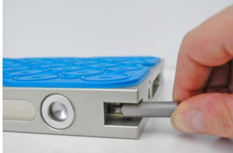
Fig. 7: Release the screws
