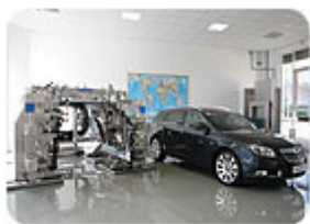
General Motors Europe was able to get the most out of the flexible match metal fixture system by using it for the sedan, coupe and wagon with limited retooling. Source: Witte and General Motors Europe
