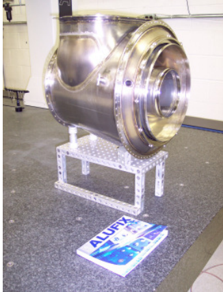
Photo 1: Turboshaft mounted on standard Alufix 25 components for CMM measuring
