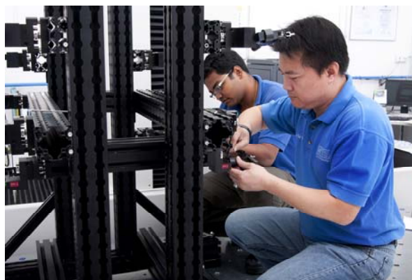
Photo left: Aluquick-fixture for car sheetmetal-parts left/right Photo right: Mounting of Aluquick components
