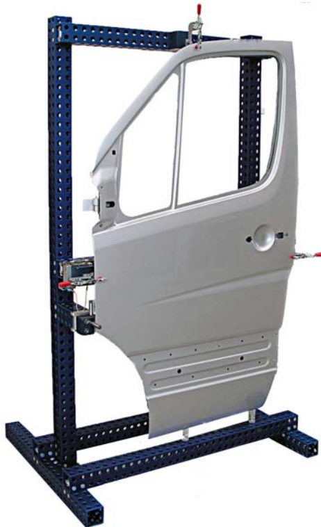
Photo left: Alufix ECO fixture mounted with car door. The blue colour makes it easy to distinguish from Alufix Classic
