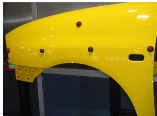
Picture: Laser pointer detects the target positions for Fixinspect accessories on a fender
