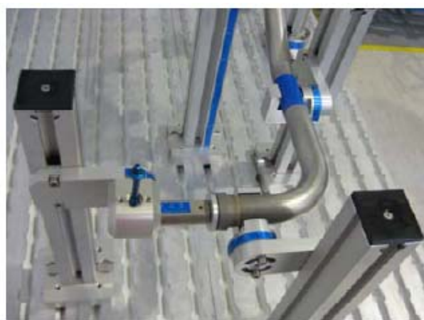
Photo left above: Aluquick fixture showing irregular shaped pipe mounted for measuring..
