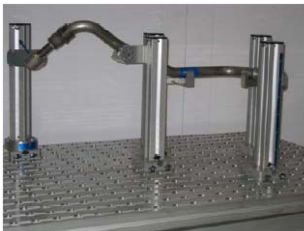
Photo left above: Aluquick fixture showing irregular shaped pipe mounted for measuring..
