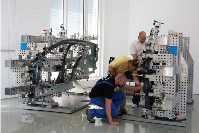
A 53 Mounting side panels: Staff mounting car side panels on to the fixture
