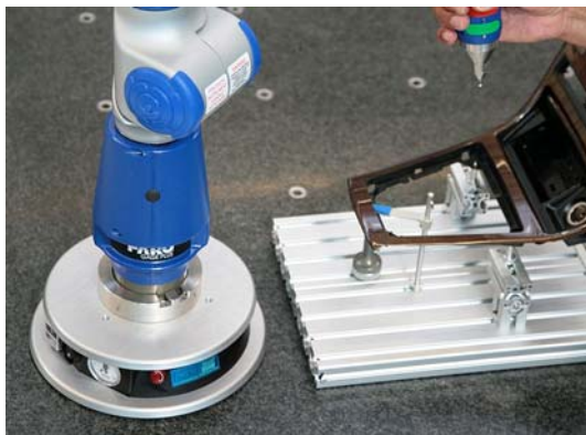
Pictures: Vacuum-Disc for mounting mobile measuring arms
